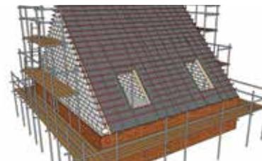
Installation of roofing membrane and tiling battens.
