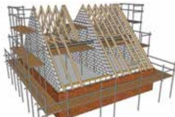
Installation of loose rafters, forming of dormer and roof window openings.
