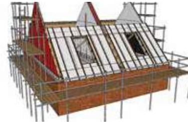
The spandrel top hats are installed and the remainder of the panels can be fitted. The optional ceiling timbers were also installed. Not bad for a mornings work! ✓
